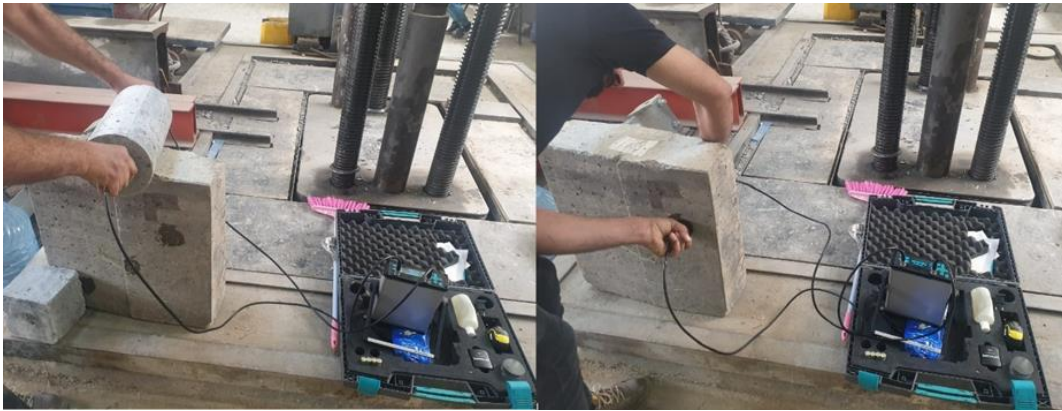
Figure 2. UPV test for concrete block and cylinder specimens
