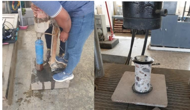
Figure 3. Concrete core sampling and testing
