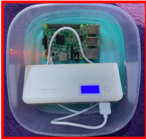
FIGURE 8 Structure of base station unit
