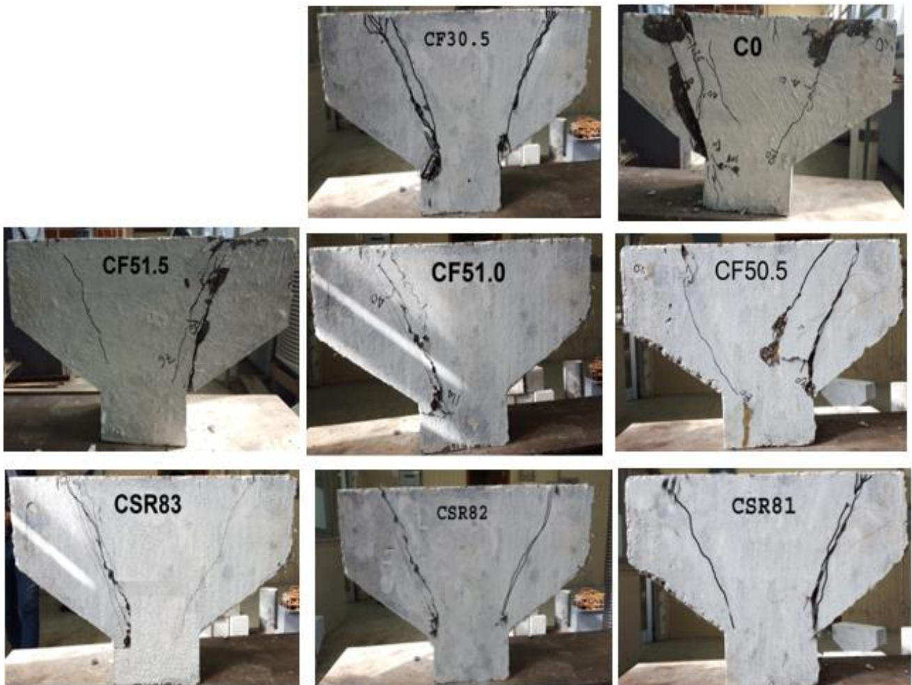
Figure 8. Typical crack pattern of some tested specimens
