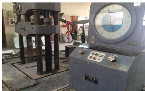
Fig. (3-8) Universal hydraulic machine TORSEE
