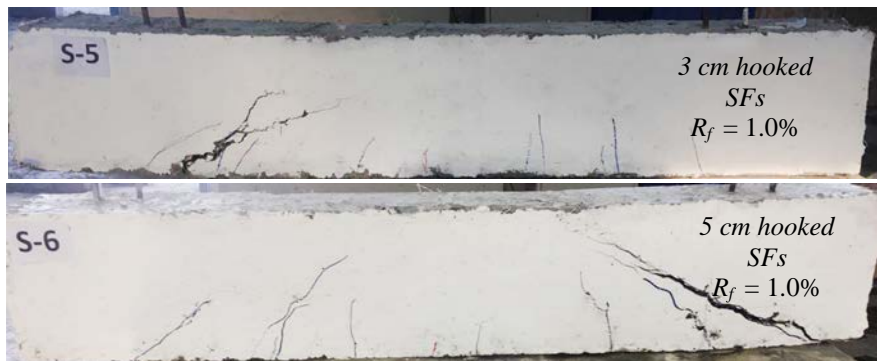
(f) Beams S5 and S6 (with 1.0% 3 cm and 5 cm hooked SFs, respectively)
