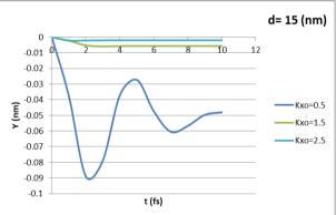
**Figure 5.** Time dependence of the average value  $\overline{y}(t)$  for  $\alpha$ =1 and  $\beta$ =I, in the transversal orientation,  $k_{yo}$ =0, (a) d=5 nm, (b) d=10 nm, (c) d=15 nm.
