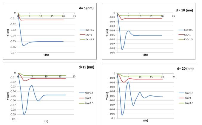
**Figure 2.** Time dependence concerning the average value of  $\overline{y}(t)$  for  $\alpha$ =1 and  $\beta$ =0, ( $\alpha$ ) in transversal orientation,  $k_{yo}$ =0, ( $\alpha$ ) d=5 nm, ( $\alpha$ ) d=10 nm, ( $\alpha$ ) d=15 nm, ( $\alpha$ ) d=15 nm, ( $\alpha$ ) d=20 nm
