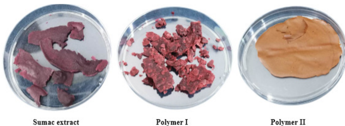
Fig. 1 : Colure change according to the polymerization with I) citric acid II) folic acid.
