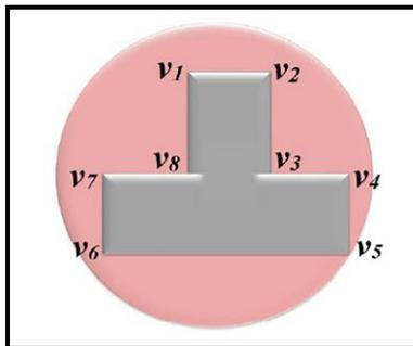
Fig.5. the complete virtual circle of the obstacle [21].
