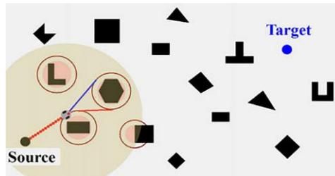
Fig.6. the shortest tangential path of the obstacle virtual circle [21].
