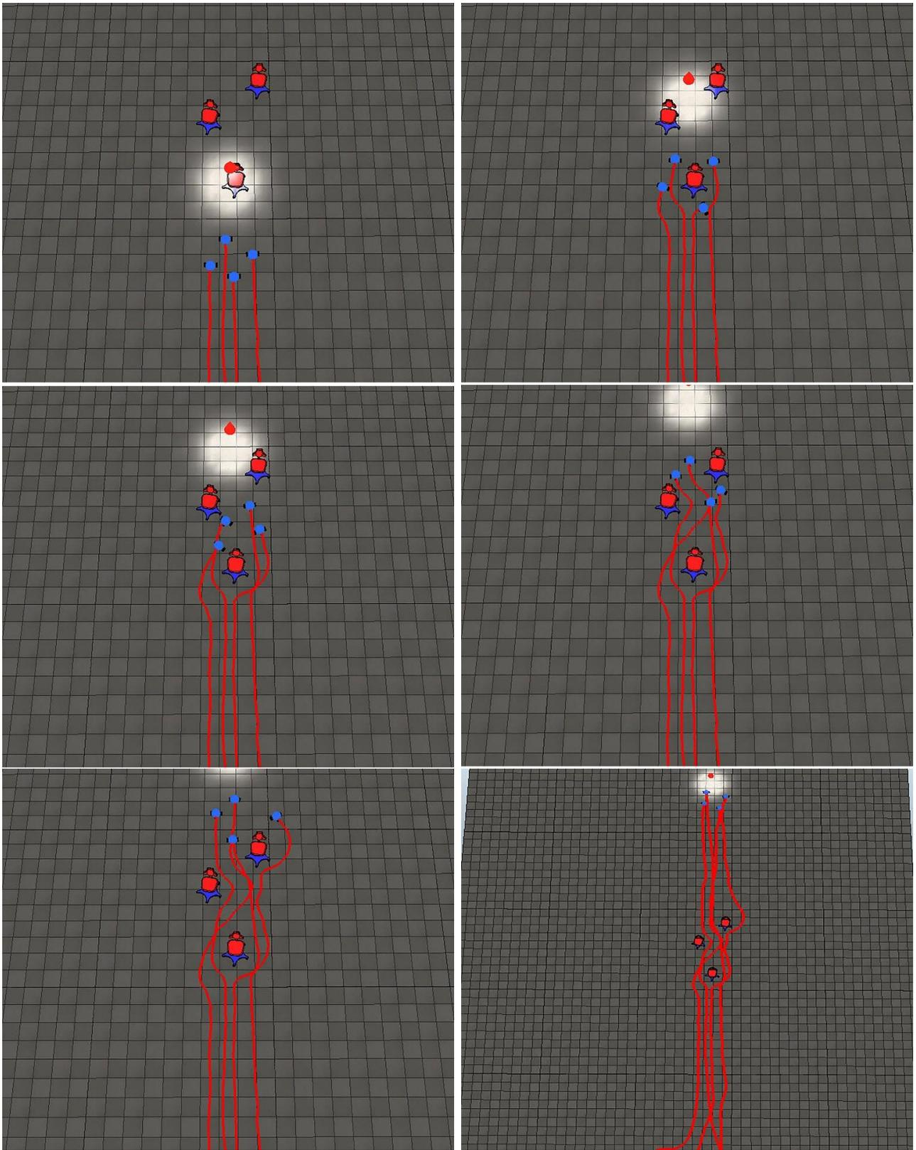
**Fig.14.** Straight-line pattern with obstacles avoidance according to the dynamic model (parameters evaluated by the physical structure of the robot)
