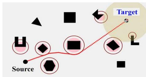
Fig.7. the virtual circular shapes of the obstacles [21].
