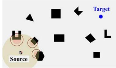
Fig.2. the detected obstacles by the sensing zone of the robot [20].
