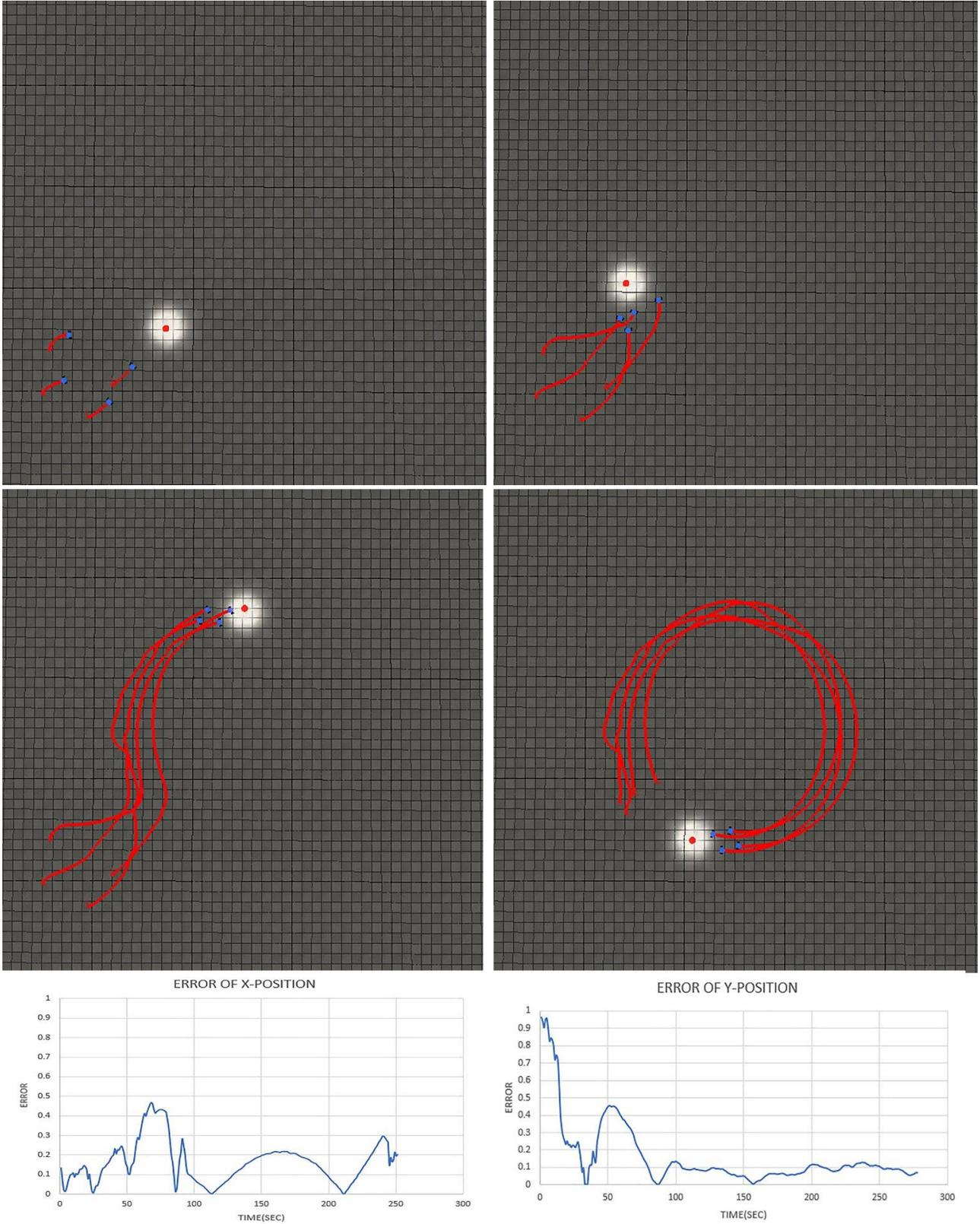
**Fig.11.** The circular pattern according to the dynamic model (parameters evaluated by the least parameter estimation method).
