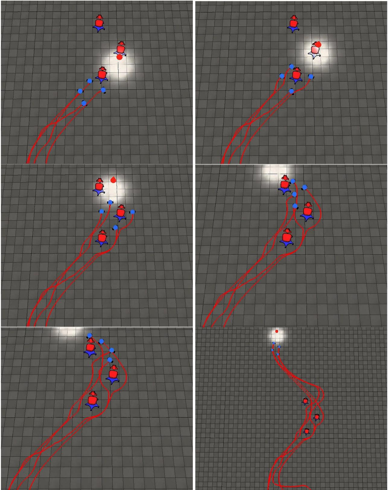
**Fig.19.** the zigzag pattern with obstacles according to the dynamic model (parameters evaluated by the least parameter estimation method).
