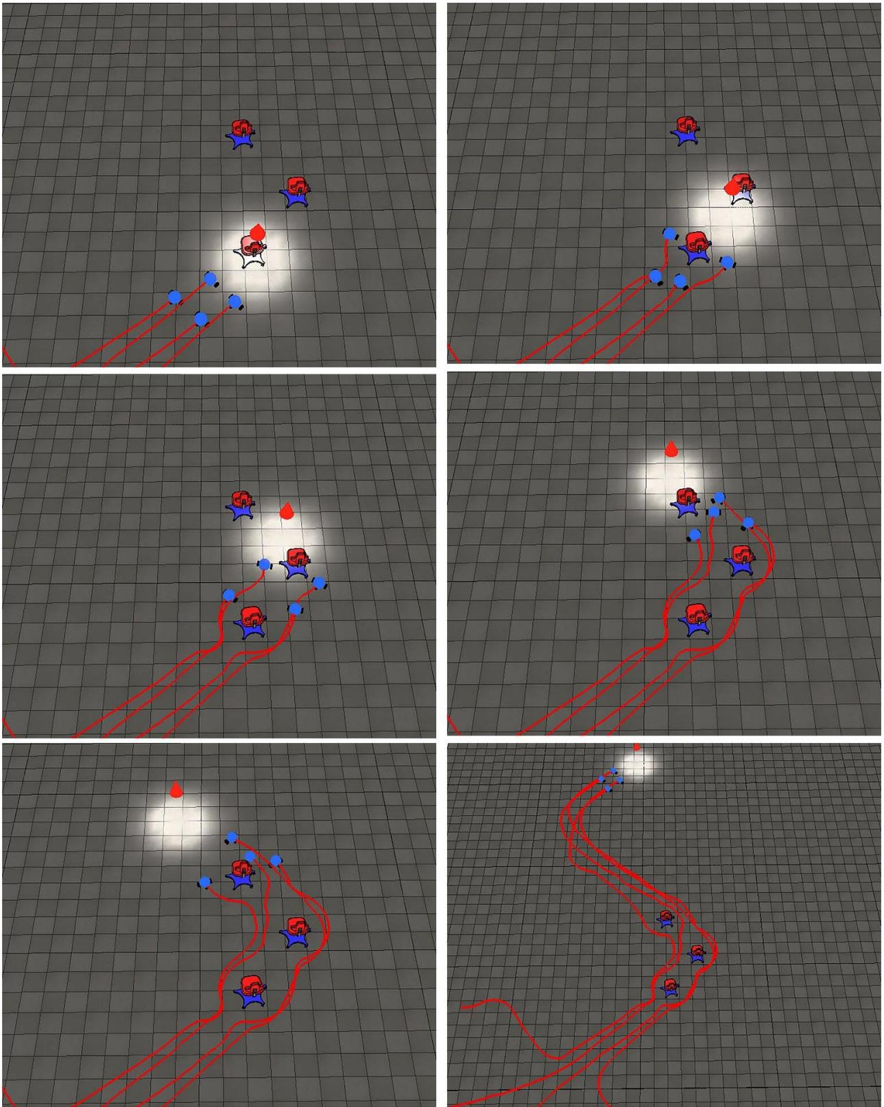
**Fig.18.** the zigzag pattern with obstacles according to the dynamic model (parameters evaluated by the physical structure of the robot)
