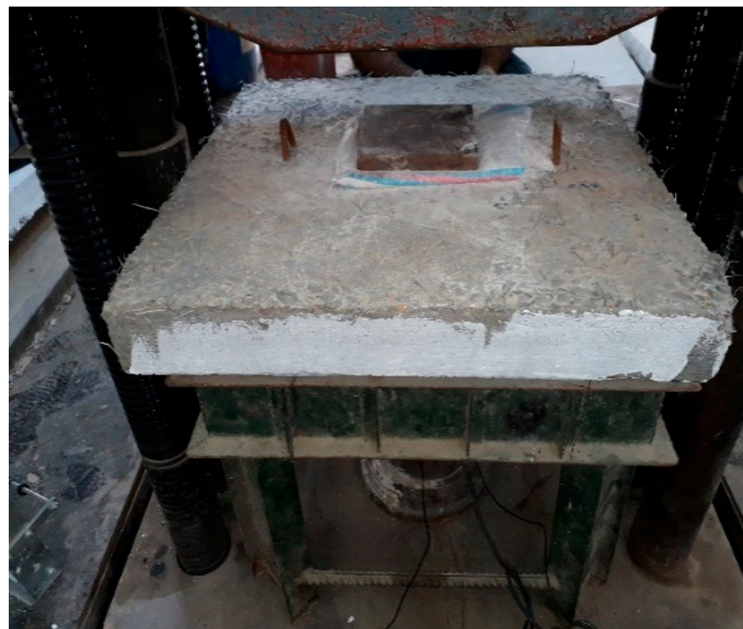
Figure 6. Slab set up for test.
