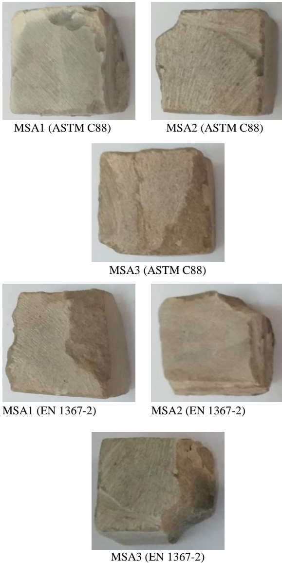
Fig4. Specimens from the Muthanna-Salman Area region after testing.
