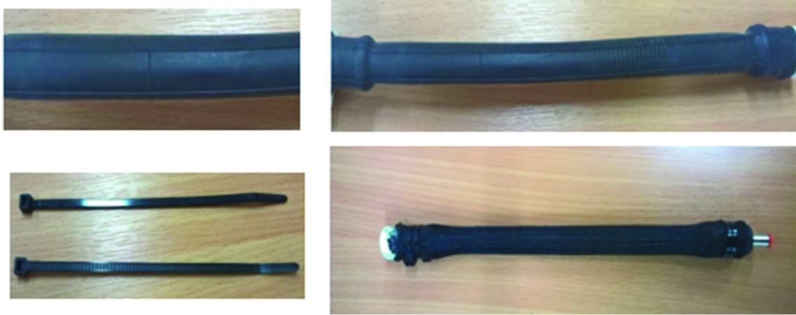
*Figure 3.5 Prototype of a contractor PMA used in the characterization experiments*
