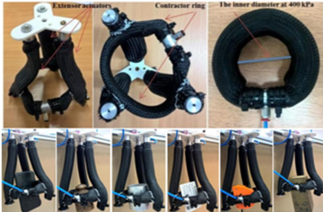
*Figure 3.27 The structure of the extension-circular gripper also showing its ability to grasp objects of different shapes and center axis [32]*
