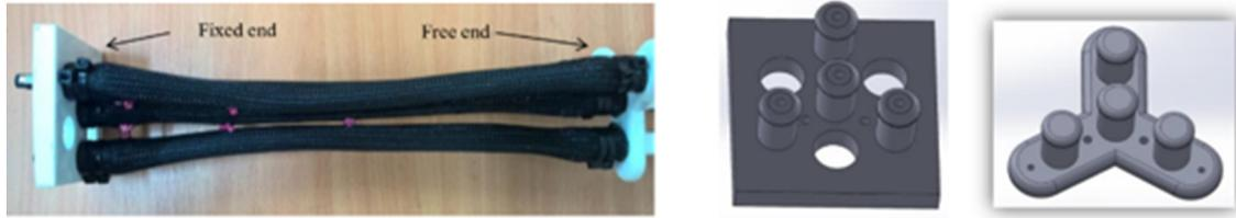
Figure 3.11 Prototype and mechanical design of the fixed and free end of the four parallel actuators for the continuum arm [30]
