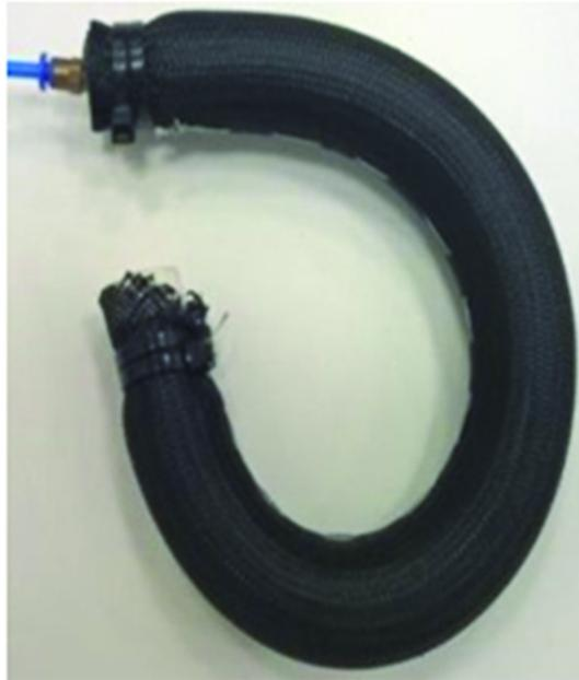
*Figure 3.20 An EBPMA at bending when pressurized at 300 kPa
