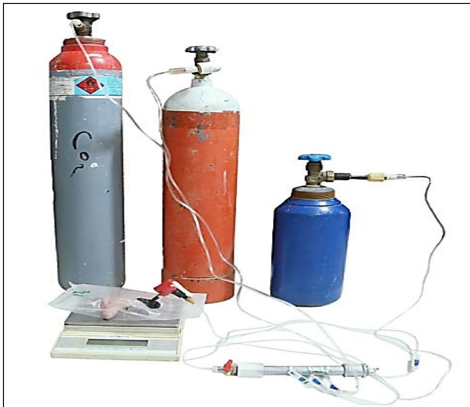
Fig. (2): Photo of the gas pumping system in meat bags.
