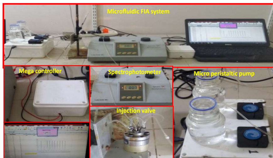
Fig. 1a. Home-made microfluidic FI spectrophotometric system which was designed
