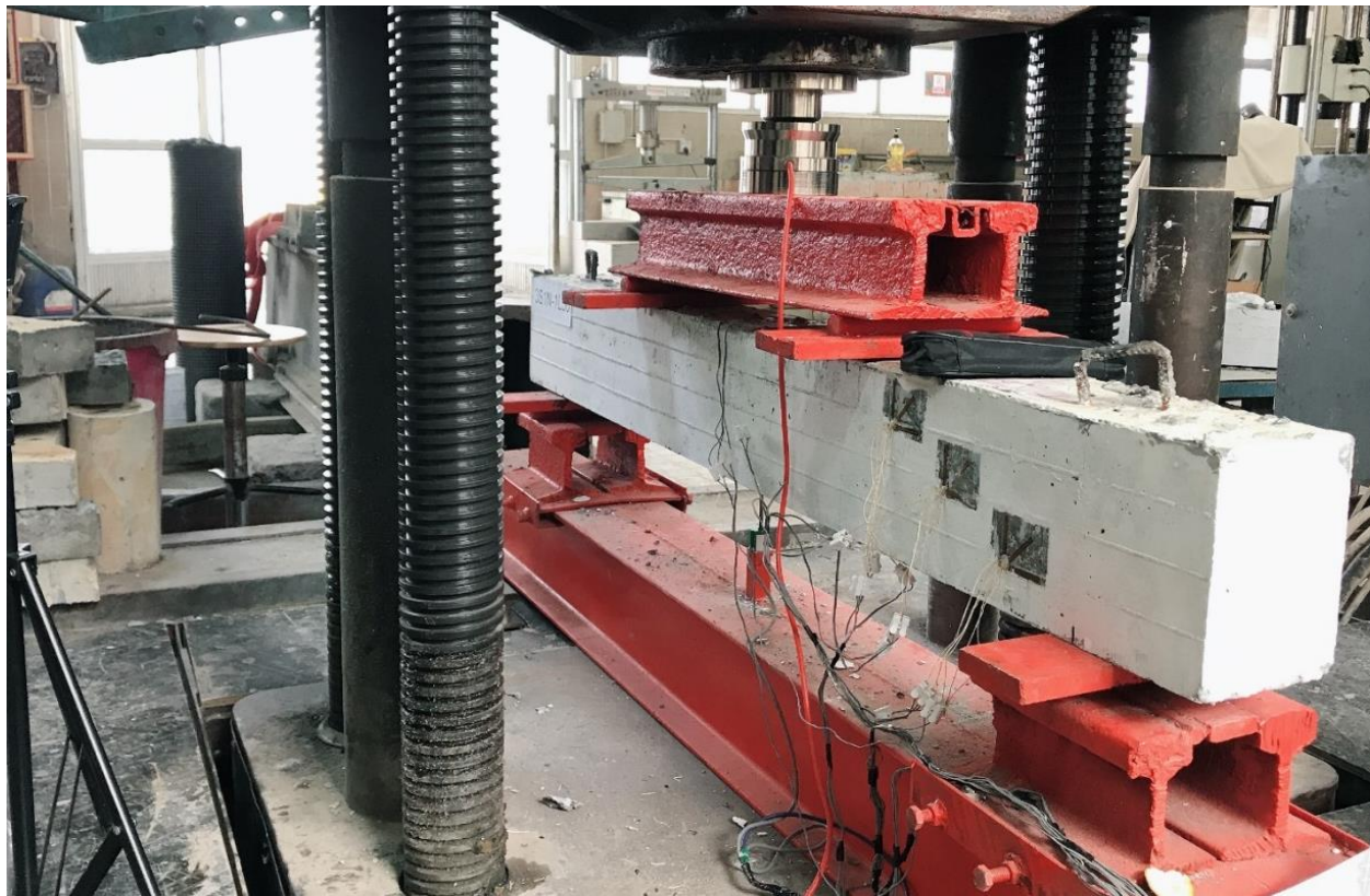
Fig. 2 The experimental set-up for the reinforced two-layer beam.
