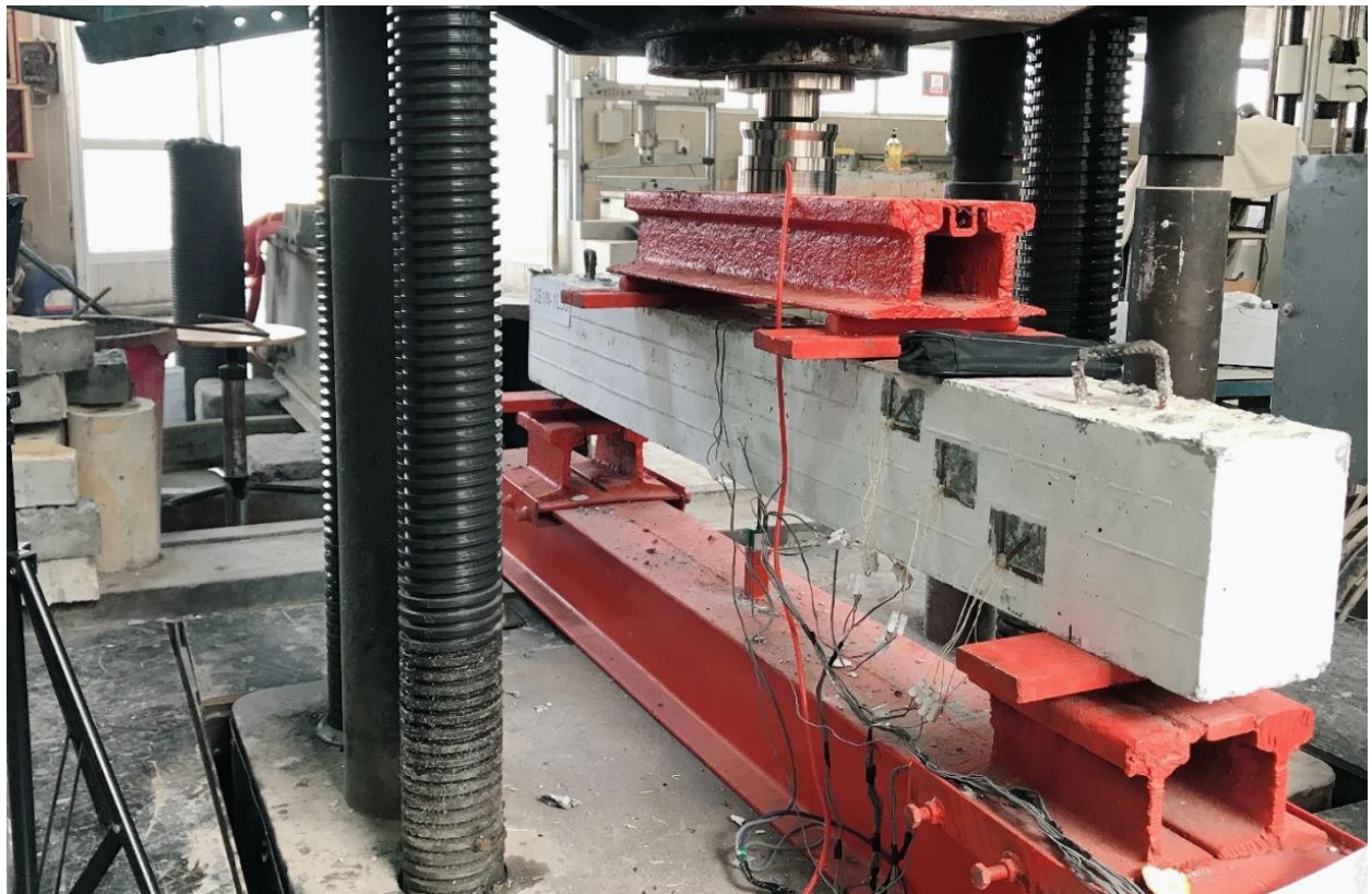
Fig. 2 The experimental set-up for the reinforced two-layer beam.
