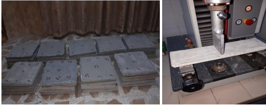
Figure 3. Sample and Flexural test device
