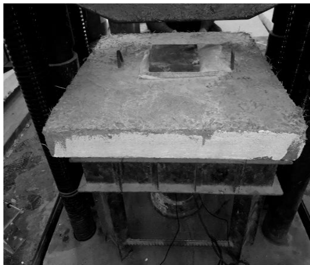
Figure 6. Slab set up for test.
