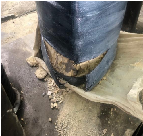
Sample with CFRP during the test
