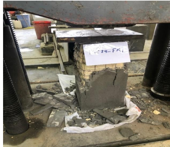
Sample with mesh wire during the test
