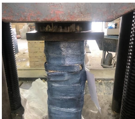
Sample with CFRP during the test
