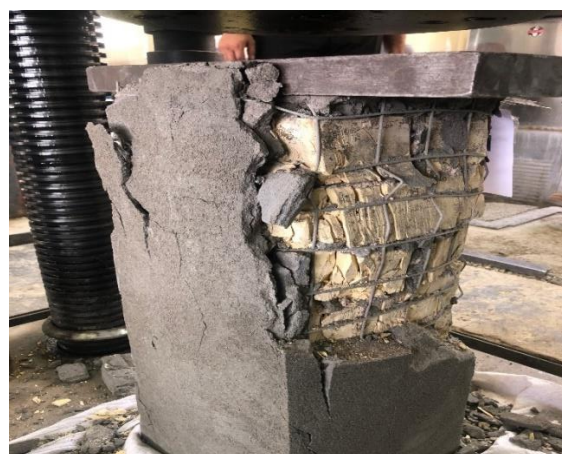
Sample with mesh wire during the test
