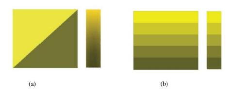
Figure 2. Schematic of material gradient (a) continues, (b) stepwise
