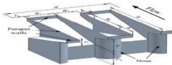
Fig.1. 3D view of the PKW (Belzner et al. , 2017))
