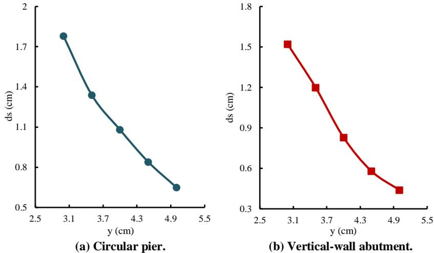
**Fig. 8. Impact of flow depth ( $y$ ) on depth of scour ( $ds$ ).**
