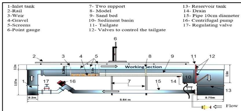
Fig. 1. Experimental flume drawing with details.
