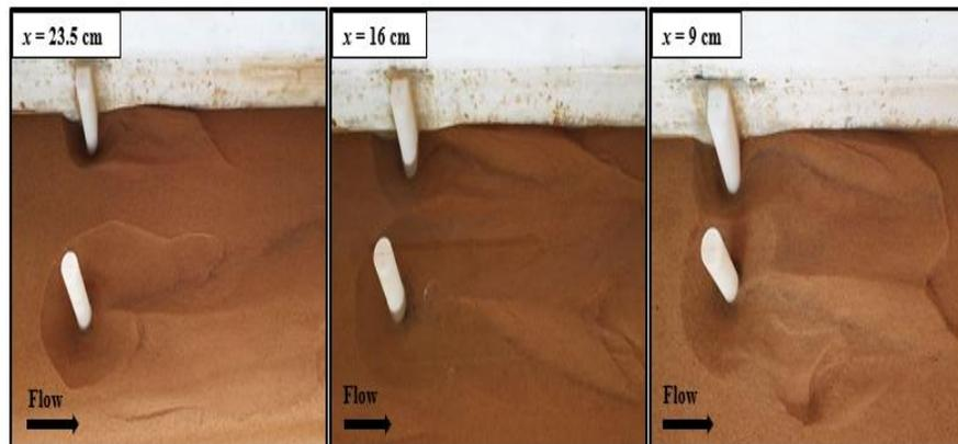
Fig. 14. Spacing variable influence amidst pier and semicircular abutment.
