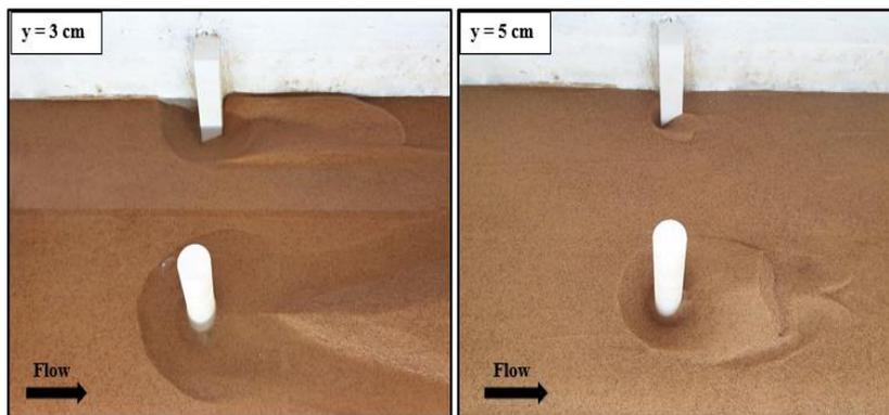
**Fig. 9. Photos that clarify flow depth effect on scouring process.**
