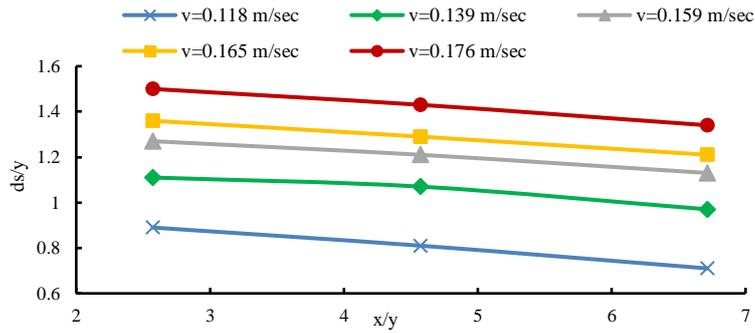
**Fig. 10.** Effect of spacing ratio ( $x/y$ ) on scour depth ratio ( $ds/y$ ) at different flow velocities and constant flow depth ( $y$ ) for circular pier.
