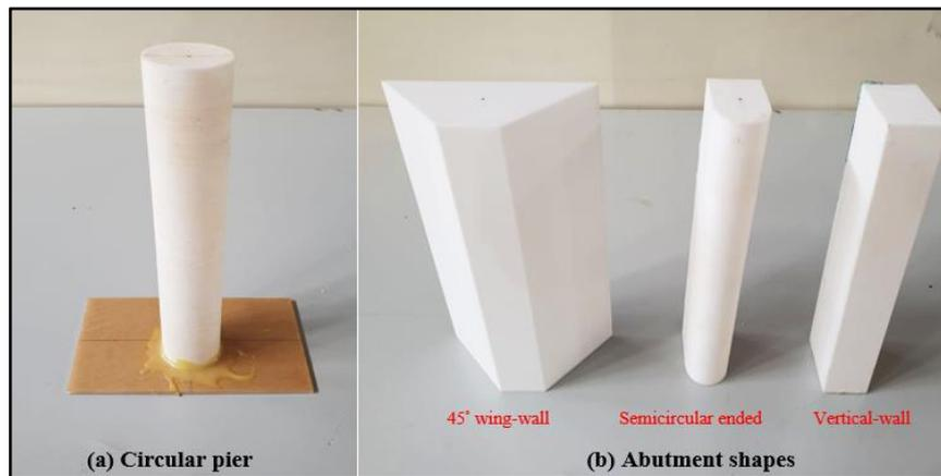
Fig. 2. The plastic models of pier and abutment.
