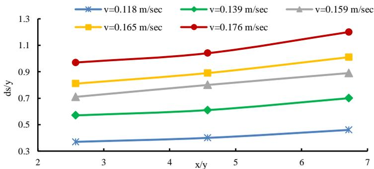
**Fig. 11.** Effect of spacing ratio ( $x/y$ ) on scour depth ratio ( $ds/y$ ) at different flow velocities and constant flow depth ( $y$ ) for vertical-wall abutment.
