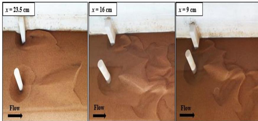
Fig. 13. Spacing variable influence amidst pier and vertical-wall abutment.
