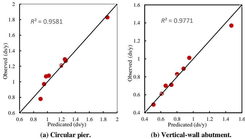
**Fig. 16. Validation of Eqs. (4) and (5) as derived from SPSS program with experimental data.**
