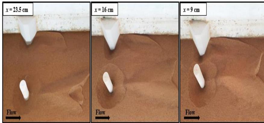
Fig. 15. Spacing variable influence amidst pier and 45° wing-wall abutment.
