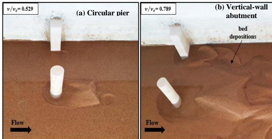
Fig. 5. The impact of flow intensity ( $v/v_c$ ) on scouring development ( $ds/y$ ).
