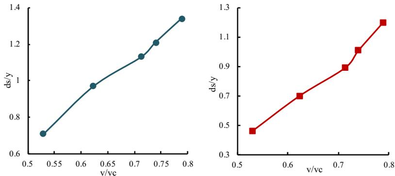
Fig. 4. Intensity of flow ( $v/v_c$ ) effect on scour depth at constant flow depth.
