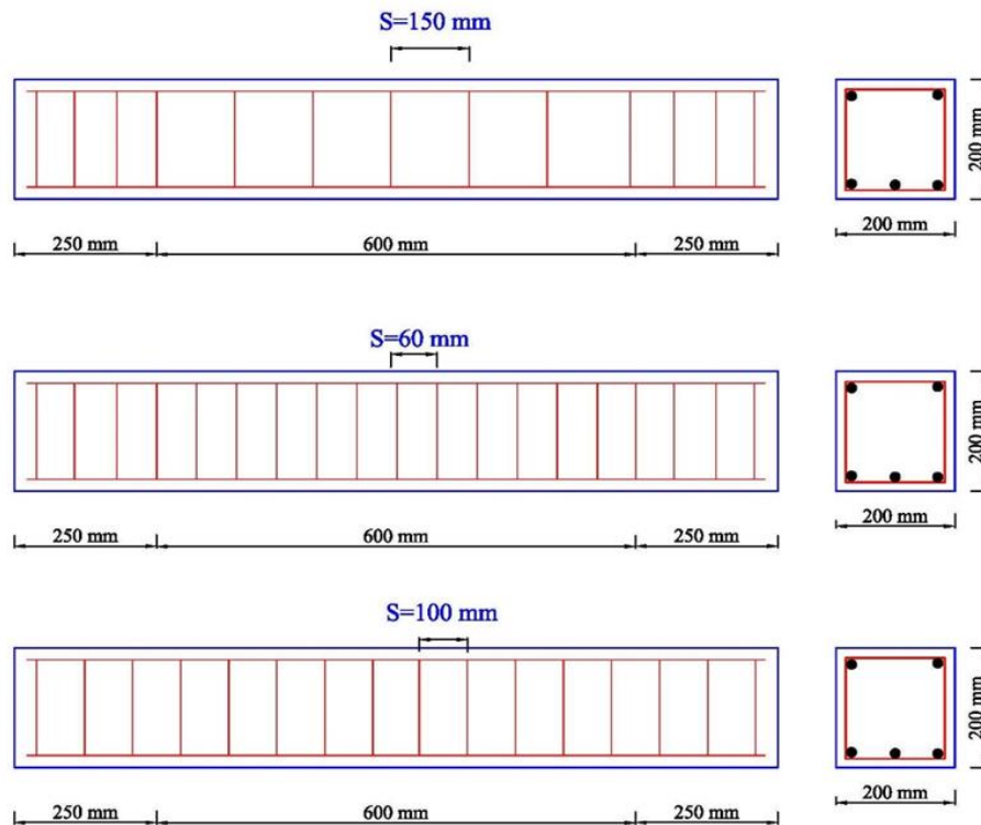
Figure 2. Beam Specimen Geometry Details
