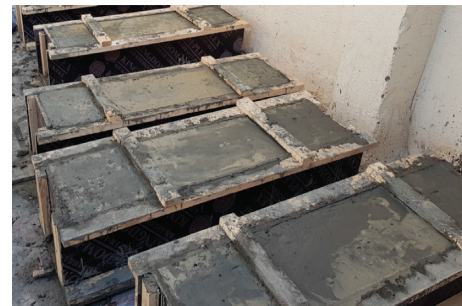
FIGURE 2: Casting of concrete specimens.
