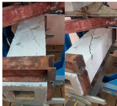
FIGURE 6: Crack pattern of beam BM0.
