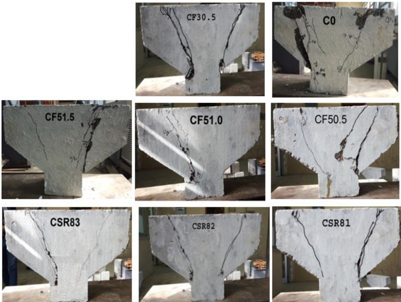
Figure 8. Typical crack pattern of some tested specimens
