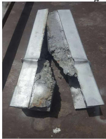
Figure 13: Failure mode of specimen SHS9
