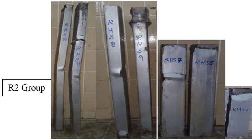
Figure 12: failure mod of S3 and R2 groups specimens.
