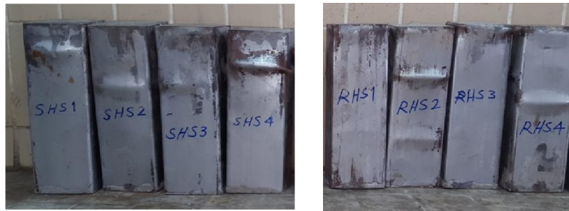
Figure 6: Failure shape of the specimens after testing
