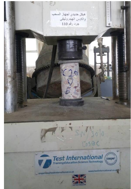
Fig. 2. Core sample in crushing machine.
