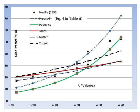
Fig. 7: Relation between ultrasonic pulse velocity and concrete compressive strength based on the paper proposed model and researchers model.
