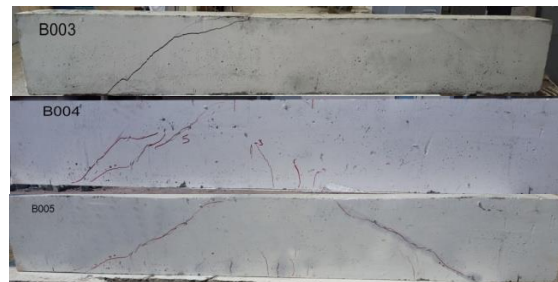
Figure 5: Crack pattern of group one ferrocement beams.
