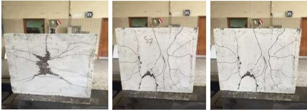
Fig. 9: Slab after testing
