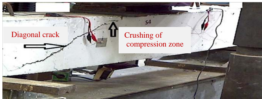
Fig. 5 Diagonal crack in an SF-reinforced concrete beam
