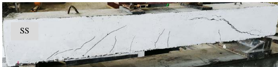
(a) Beam SS (with stirrups and without SFs)
