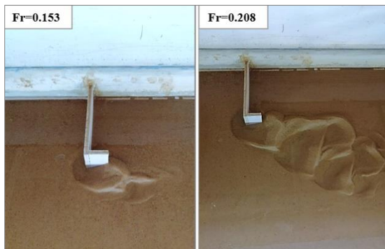
Fig. 10. Photos that clarify the effect of Froude number (Fr) on the ratio of scour depth development ( ds/h_o ) for single L-shape Groyne.
