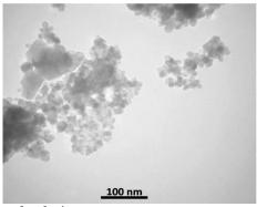
Figure 4. TEM micrograph of NiFe<sub>2</sub>O<sub>4</sub>.
