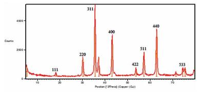
Figure 2. XRD spectrum of NiFe<sub>2</sub>O<sub>4</sub>.
