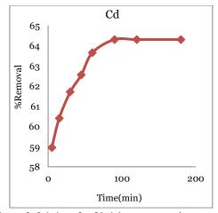
Figure 7. Effect of contact time on adsorption of pb(II) and Cd(II) ions onto NiFe<sub>2</sub>O<sub>4</sub>.
