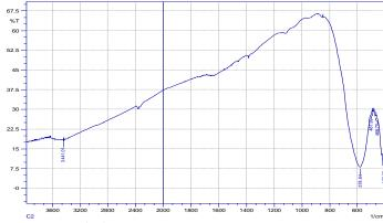
Figure 1. FT-IR spectra of NiFe<sub>2</sub>O<sub>4</sub>.
