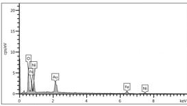
Figure 5. EDX spectra of NiFe<sub>2</sub>O<sub>4</sub>.
