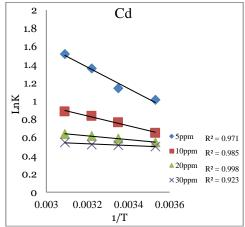
Figure 12. Plot of lnK against 1/T for adsorption of Pb(II) and Cd(II) ions on NiFe<sub>2</sub>O<sub>4</sub> nanoparticles.
