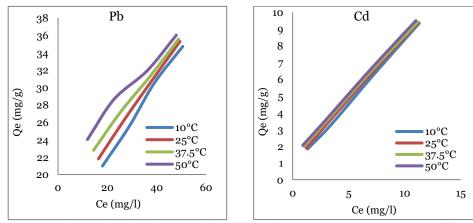
Figure 9. Adsorption isotherm of Pb(II) and Cd (II) on NiFe<sub>2</sub>O<sub>4</sub> at different temperatures.
