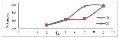
Figure 8. Effect of pH on Pb(II) and Cd(II) adsorption on NiFe<sub>2</sub>O<sub>4</sub>.
