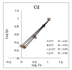
Figure 10. Linear form of Freundlich isotherms of Pb(II) and Cd(II) on NiFe<sub>2</sub>O<sub>4</sub> at different temperatures.
