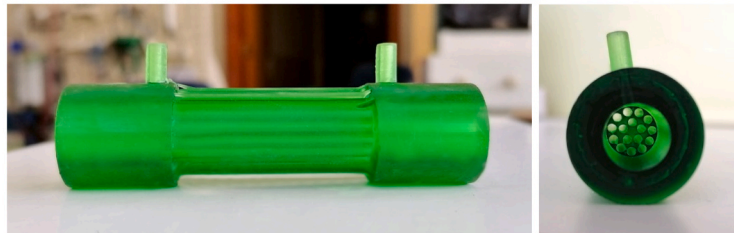
(c) LM fully casted by high precision 3D printing, circular tubes and divergent pressure taps
