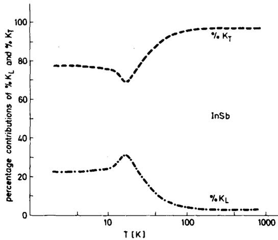
Fig. 2. The percentage contributions  $\% K_T$  and  $\% K_L$  towards the total lattice thermal conductivity of InSb due to transverse and longitudinal phonons, respectively. Dashed and dot-dash lines represent  $\% K_T$  and  $\% K_L$ , respectively
