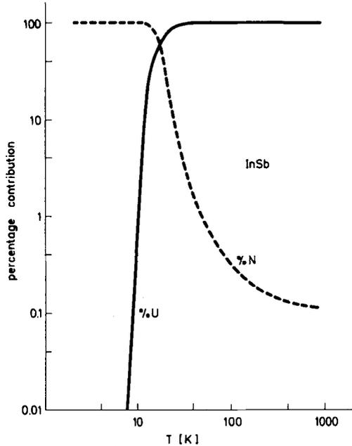
Fig. 3. The percentage contributions  $\% \tau_{3ph,N}^{-1}$  and  $\% \tau_{3ph,U}^{-1}$  processes towards the  $\tau_{3ph,T}^{-1}$  for class I events for transverse phonons for InSb in the temperature range 2–800 K. Solid and dashed lines represent  $\% \tau_{3ph,U}^{-1}$  and  $\% \tau_{3ph,N}^{-1}$ , respectively
