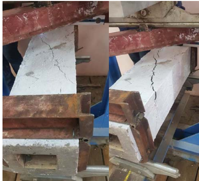
Figure 6. Crack pattern of specimen B0.
