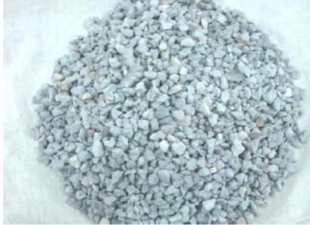
Figure 2. Recycled aggregates
