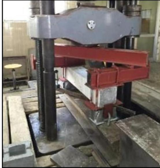
Figure 3. Test setup for beams
