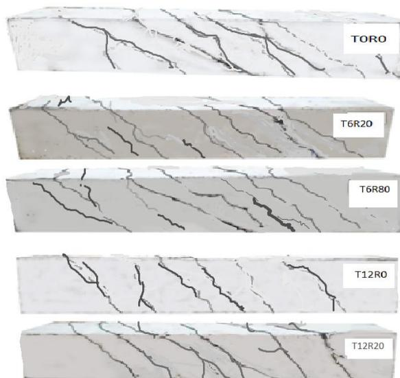
Figure 7. Cracks pattern of all tested beams
