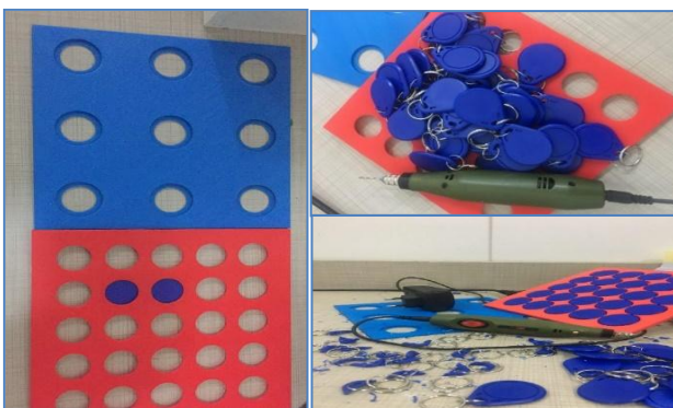
Fig .7. Different types for the lower part of the RFID localization system (5*5 holes) and (3*3 holes).
