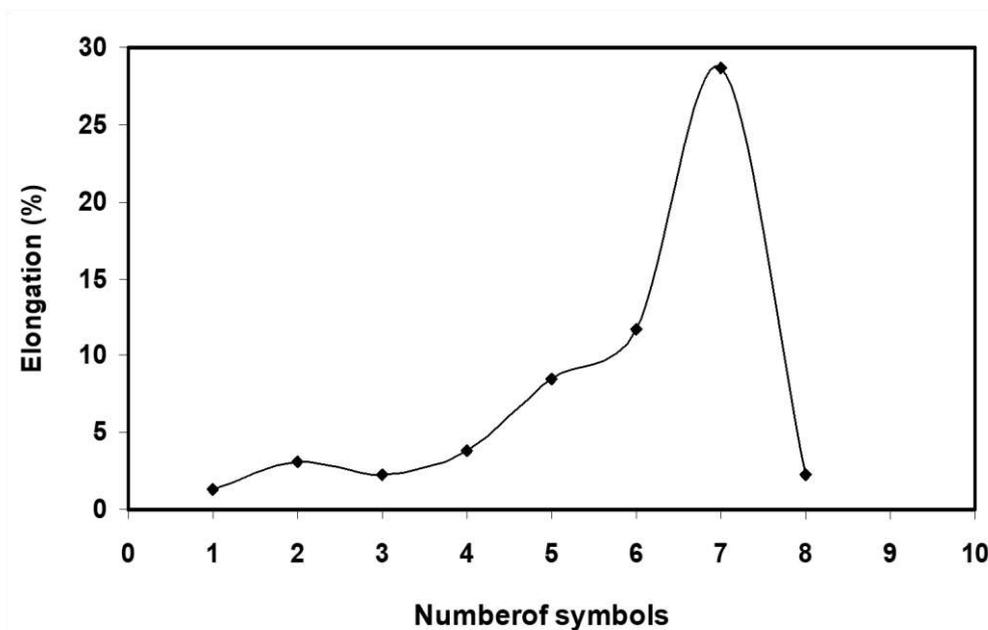
Figure (8): Elongation of rPS and, rPMMA blends with ratio of diethyl malonate.
