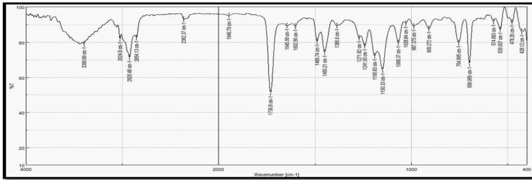
Figure (2): (FTIR) Spectroscopy of polymer blend 2.
