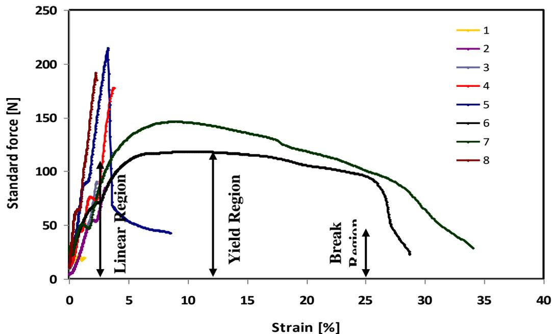
Figure (6): the stress-strain curves of polymer blends of (rPS) and (rPMMA) with different ratio (diethyl malonate).
