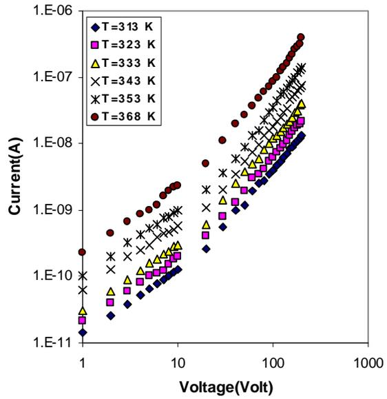
Figure(5):The (current-voltage)characteristics at different temperature range (313-368)K.
