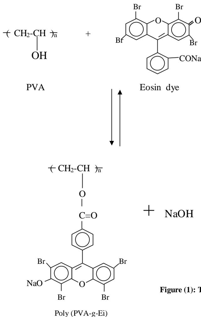
Figure (1): The diagram structure reaction of PVA-g-Ei.
