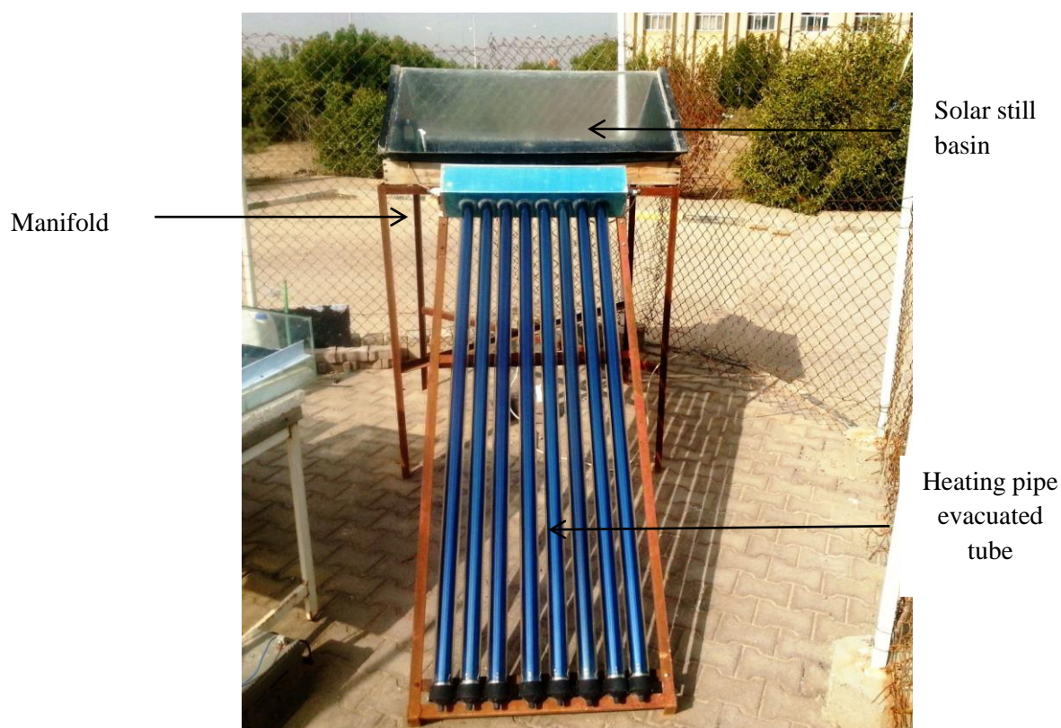
Figure 2: shows the total system of solar desalination
