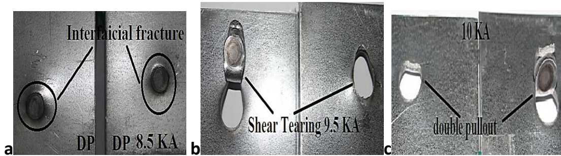
Fig (13): Failure modes of DP600/DP600 RSW: (a): Interfacial Failure mode. (b): shear tearing. (c): double pullout failure .
