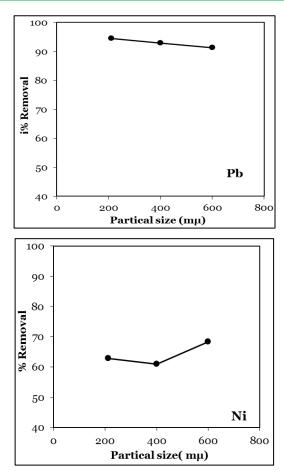
**Fig. 2.** The relationship between the percentage removal of Pb(II) and Ni (II) with the particle size of adsorbent.
