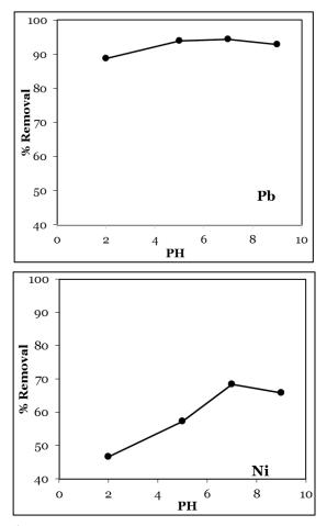
**Fig. 4.** The relationship between the percentage removal of Pb (II) and Ni (II) with PH.
