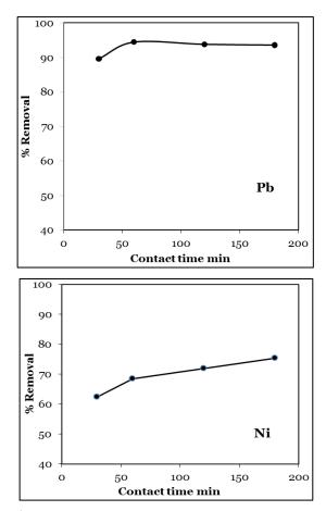
**Fig. 3.** The relationship between the percentage removal of Pb (II) and Ni (II) with time.
