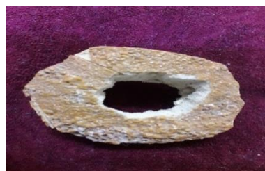
Figure 2: The coaxial shape of rice husk filled polyurethane foam
