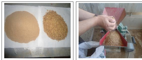
Figure 1: The rice husk before and after grinding
