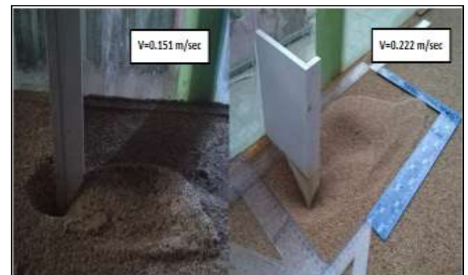
Photo 3: Effect of (V) on (d s ) development
