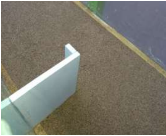
Photo 2: The L-shape groyne placed in the flume
