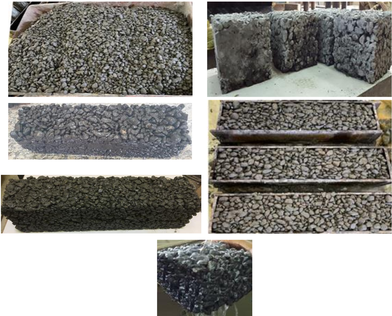
Figure 1. Casting and sampling of pervious concrete
