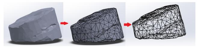
Figure 10. Converting static geometry to dynamic geometry.
