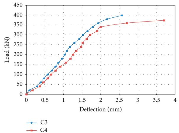
FIGURE 6: Load-deflection relationship of corbels with 0% and 50% weight fractions of replacement aggregate for concrete strength 36.2 and 35.1 MPa and  $a/d$  ratio 0.5.
