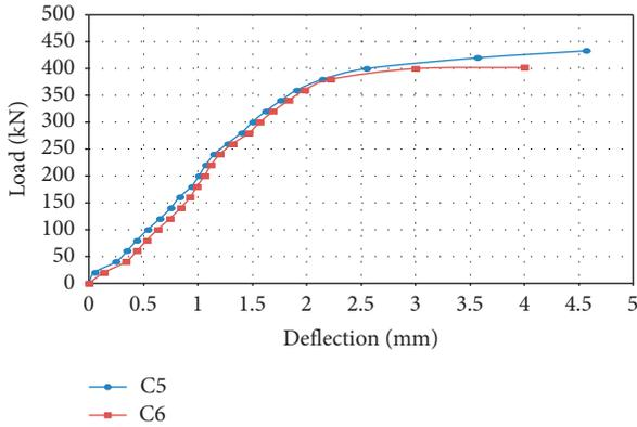
FIGURE 7: Load-deflection relationship of corbels with 50% and 100% weight fractions of replacement aggregate for concrete strength 45.8 and 44.3 MPa and a/d ratio 0.5.
