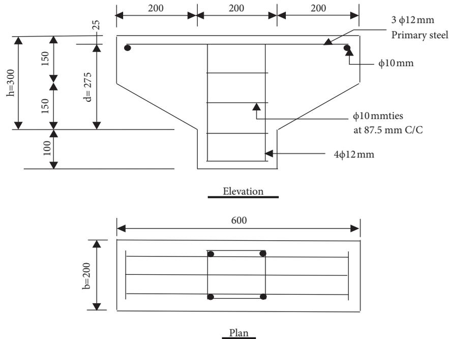
FIGURE 1: Details of corbels and reinforcement.
