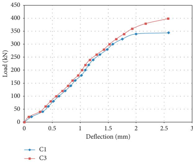
FIGURE 8: Load-deflection curve of corbels of 0% weight fractions of replacement aggregate for concrete strength 28.2 and 36.2 MPa and a/d ratio 0.5.
