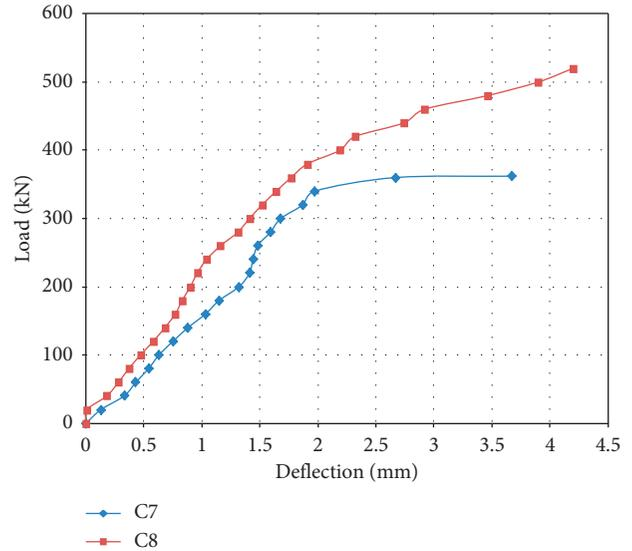
FIGURE 10: Load-deflection curve of corbels with 50% weight fractions of replacement aggregate for concrete strength 29.4 and 45.6 MPa and a/d ratio 0.35.
