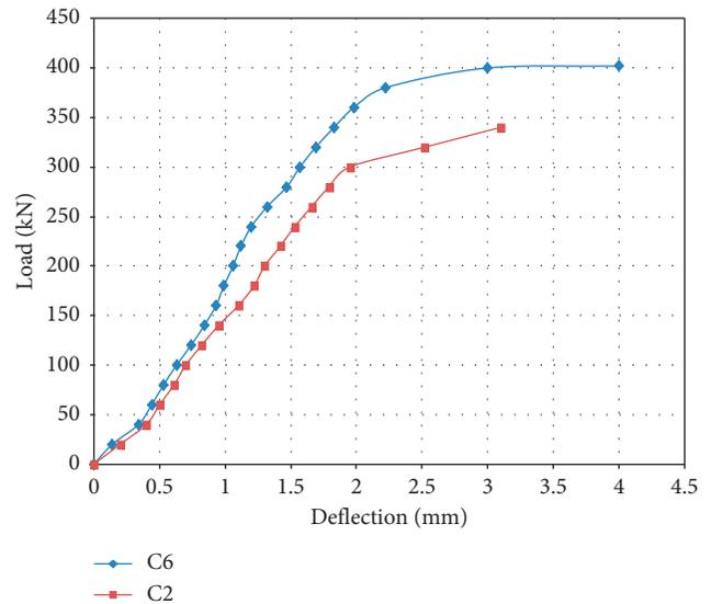
FIGURE 11: Load-deflection curve of corbels with 100% weight fractions of replacement aggregate for concrete strength 28 and 44.3 MPa and a/d ratio 0.5.
