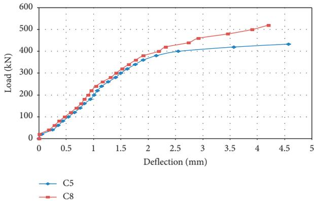
FIGURE 12: Load-deflection curve of corbels with concrete strength 45.8 and 45.6 MPa and weight fractions of replacement aggregate 50% and  $a/d$  ratio 0.5 and 0.35.
