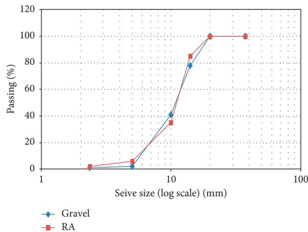
FIGURE 2: Natural coarse and recycled aggregate grading curves.
