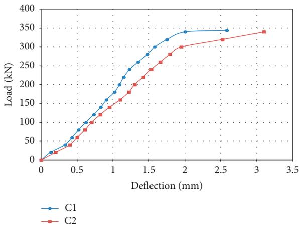
FIGURE 5: Load-deflection relationship of corbels with 0% and 100% weight fractions of replacement aggregate for concrete strength 28.2 and 28.0 MPa and  $a/d$  ratio 0.5.
