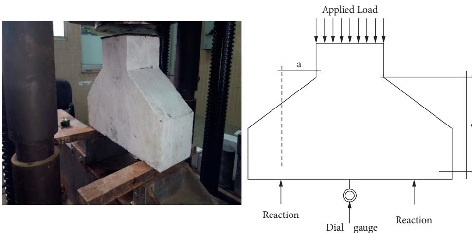
FIGURE 3: Loading arrangement of corbels.
