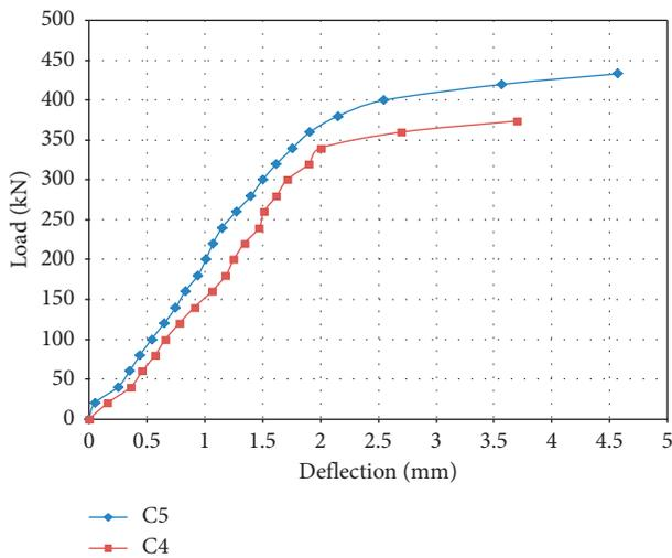
FIGURE 9: Load-deflection curve of corbels with 50% weight fractions of replacement aggregate for concrete strength 35.1 and 45.8 MPa and a/d ratio 0.5.
