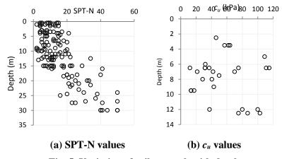
Fig. 5. Variation of soil strength with depth.
