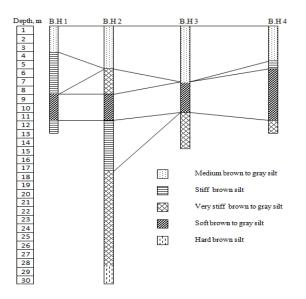
Fig. 3. Subsurface soil conditions through boreholes 1, 2, 3 and 4.
