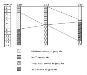
Fig. 4. Subsurface soil conditions through boreholes 6, 5 and 4.
