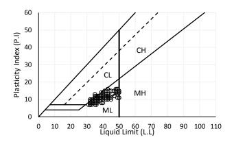
Fig. 7. Plasticity chart for Ammarah soil.
