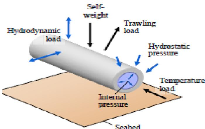
Figure 5: Typical exerted loads on the free-span of a submarine Pipeline (Kristain, 2008).
