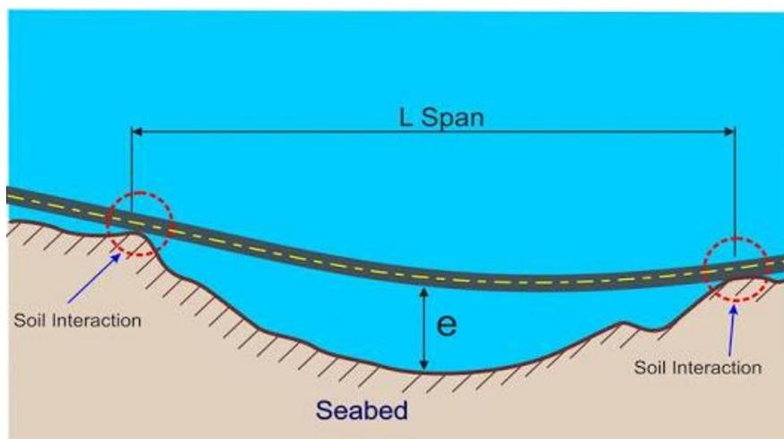
Figure 1. span performed on seabed
