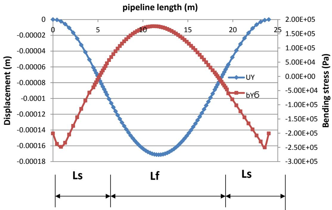
Figure 9. Displacement ( $U_Y$ ) and Bending stress ( $\sigma_{bY}$ ) configurations along total length of pipeline
