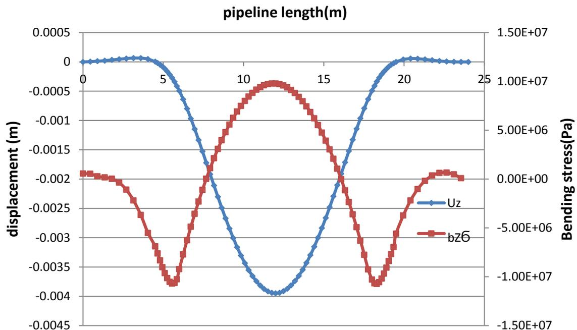
**Figure 10. Displacement ( $U_z$ ) and Bending stress ( $6_{bz}$ ) configurations along total length of pipeline**
