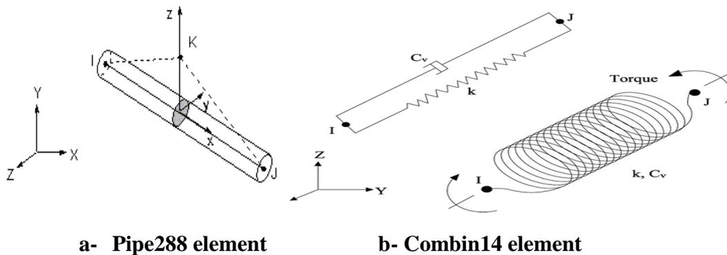
Figure 2: elements used in the Ansys Model
