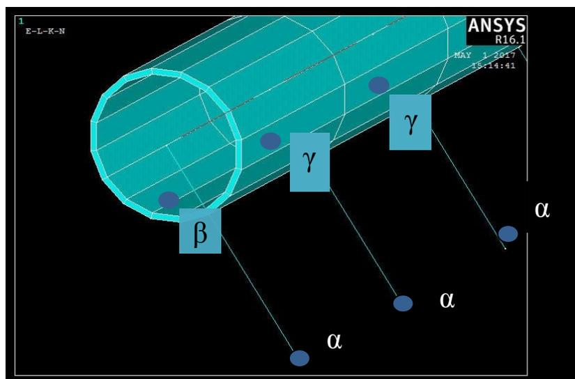
Figure 4. Boundary conditions in the ANSYS Model
