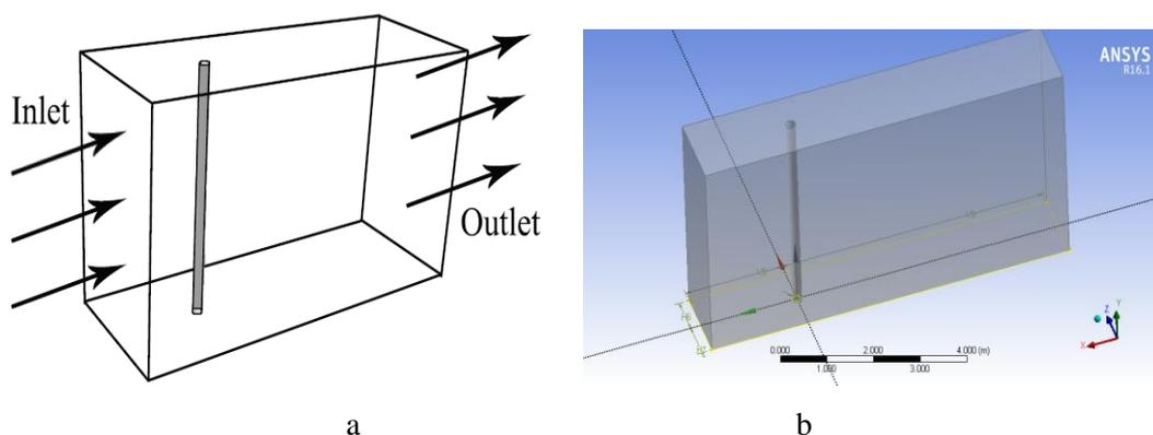
Figure 2 a) sketch of 3D fluid domain. b) Ansys 3D fluid domain.
