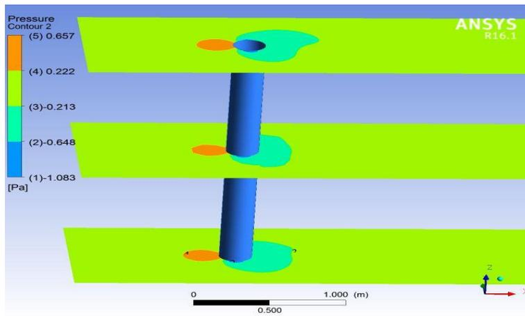
**Figure 8** Pressure distribution around Riser at  $z = 0\text{m}$ ,  $z = 1.1\text{m}$  and  $z = 2.2\text{m}$
