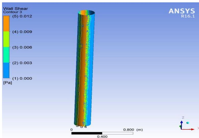
**Figure 7** Shear stress contour of Riser's wall.
