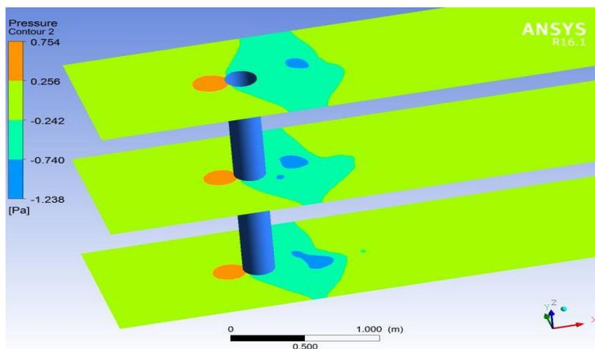
**Figure 13** Pressure distribution around Riser at  $z = 0\text{m}$ ,  $z = 1.1\text{m}$  and  $z = 2.2\text{m}$
