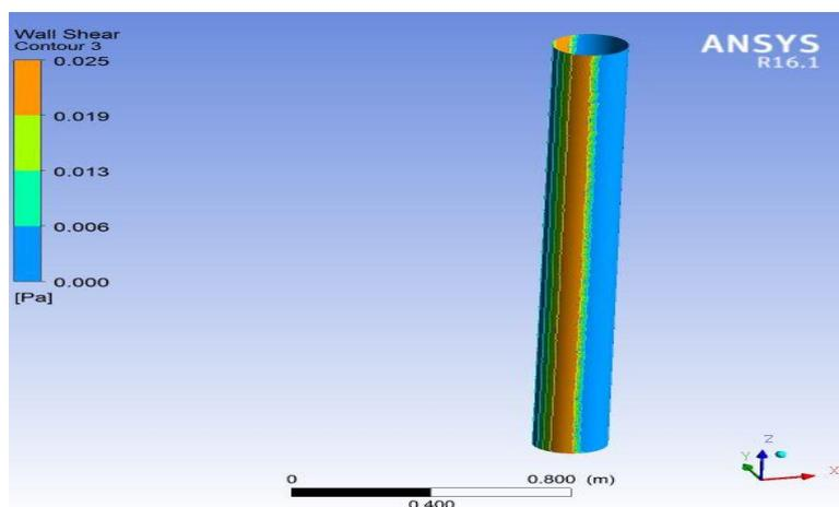
**Figure 12** Shear stress contour of Riser's wall.
